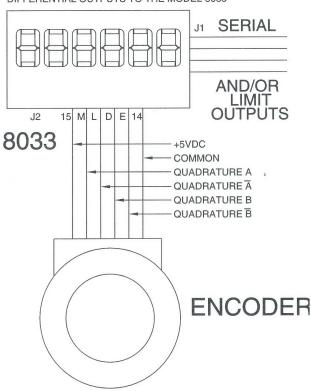
THE MODEL 8033-11-19 WILL COUNT IN QUADRATURE UP AND DOWN AND DISPLAY A NEGATIVE SIGN WHEN THE COUNT GOES THROUGH ZERO. EXCITATION VOLTAGE OF 5VDC AT 150 MA IS ALSO PROVIDED TO POWER THE ENCODER.
