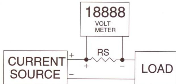
BY USING SHUNT RESISTOR RS A VOLTMETER CAN BE USED AS A AMMETER BY MEASURING THE VOLTAGE DROP ACROSS RS
